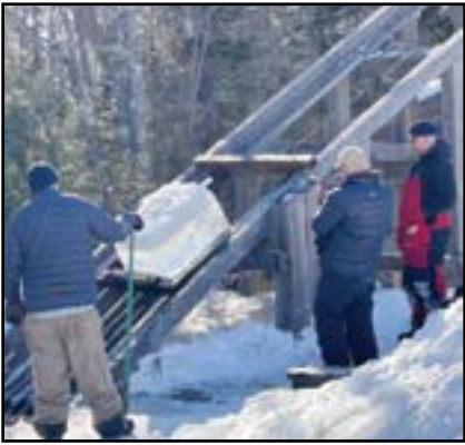
Blocks of 24-inch-square cut ice collect on the pond and are then guided with poles to the elevator incline that carries them up to be stored in the ice house.
