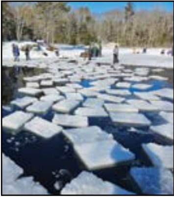
Blocks of 24-inch-square cut ice collect on the pond and are then guided with poles to the elevator incline that carries them up to be stored in the ice house.
